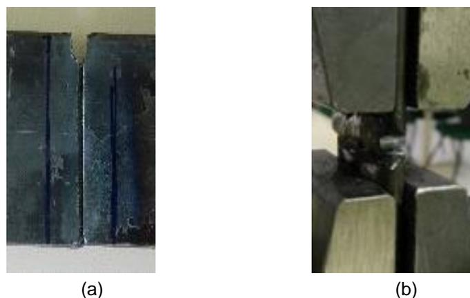
The tensile tests were carried out in an electromechanical machine model EMIC DL 10000. The load transducer has a maximum load capacity of 100 kN. The preload was  $2 \pm 2 \times 10^{-2}$  kN and the pulling speed was  $5 \text{ mm} \cdot \text{min}^{-1}$ .
