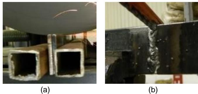
A region with a width of 13 mm was marked around the welded region (Figure 4a) so that the specimens could be precisely positioned in the fixture device for the tensile tests (Figure 4b).
