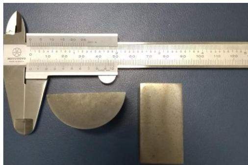
Figure 4 – Cross section and longitudinal section of the fractured tie rods. Samples removed near the fractured region.
