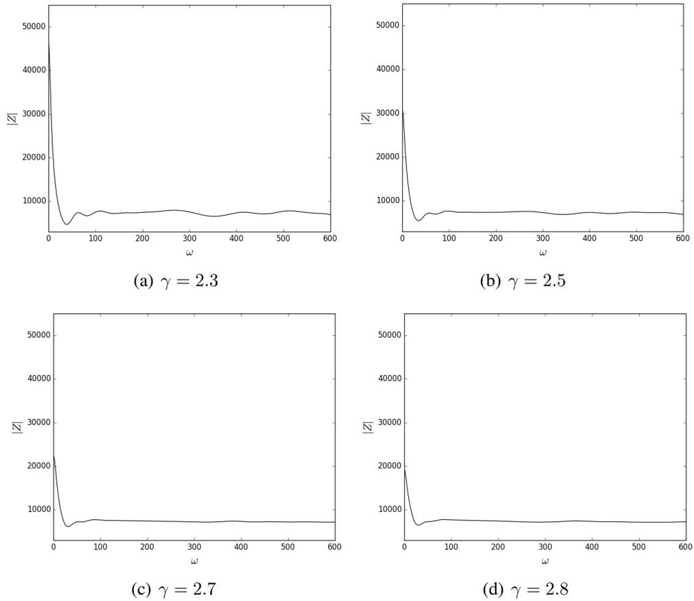
Figure 4: The input impedance module for  $\gamma = 2.3, 2.5, 2.7$  and  $2.8$ .
