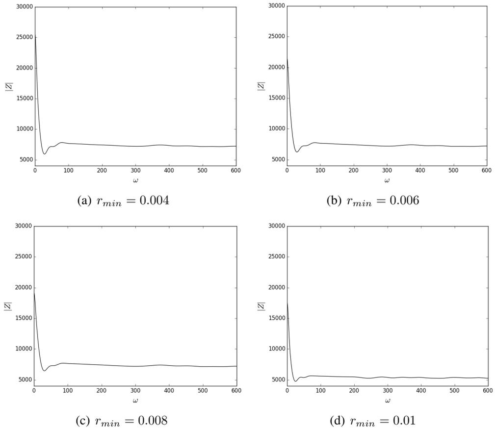
Figure 2: The input impedance module for  $r_{min} = 0.004, 0.006, 0.008$  and  $0.01$ .
